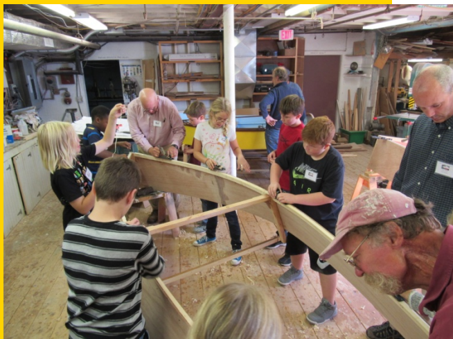
Using planes on the bottom sides of the skiff with our boat building mentors
